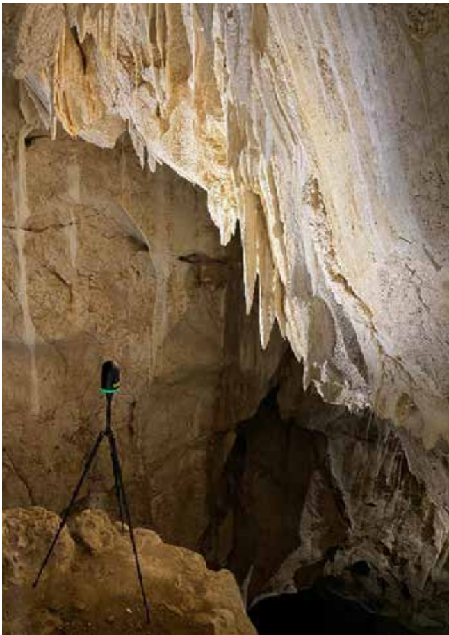
LiDAR (BLK360) setup on tripod at top of Deep Vault cave (left), and Lydia with LiDAR at bottom of Deep Vault cave (right)
