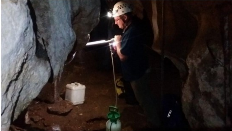
Scientist Jon Woodhead uses a custom made machine with a diamond-tipped drill to extract speleothem 'rubble' for analyzing. Credit: John Engel
